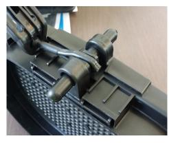
3. Ensure that the Cap Clip is correctly engaged. This may require a tap with a hammer
