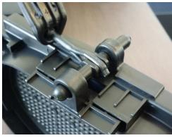
2. Insert Cap Clip in frame ready to be engaged
