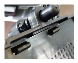
4. When the Cap Clip is correctly engaged, the 'barb' will fully protrude from the frame and lock tightly
